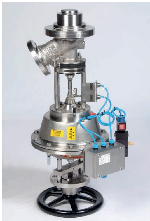
Left- a Type 25 disc-rising valve, with spring-retained short-stroke pneumatic actuator, limit-switch accessories and manual override.
