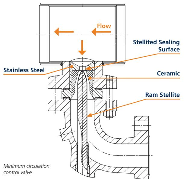
The control valve shown above was designed for a severe service pump application that included a high pressure drop ( $\Delta p$  40 bar), 30% solid contents and significant flashing.
