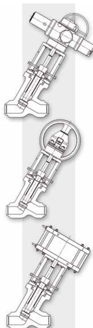
Actuator options, from top; Electric, Bevel Gearbox, Pneumatic
