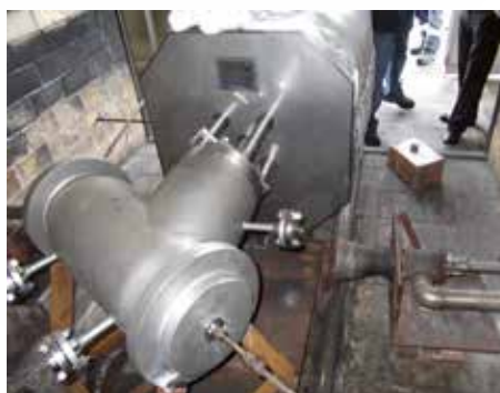
SchuF Globe Valve being fire-tested [Fire-safe Certification available, e.g. API 607]
