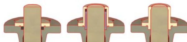
Model 28KV Radial soft seal in the valve body
