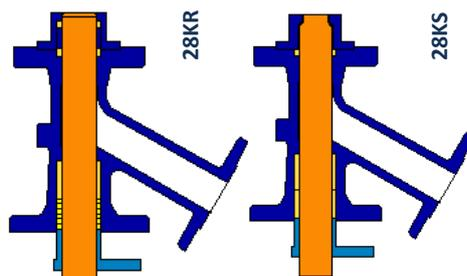
suggest either metal to metal (28KS) or radially sealed (28KR) ram type valves at the reactor outlet depending on the grade of PVC and philosophy of the customer.
