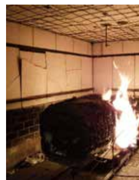
SchuF Globe Valve being fire-tested [Fire-safe Certification available, e.g. API 607]
